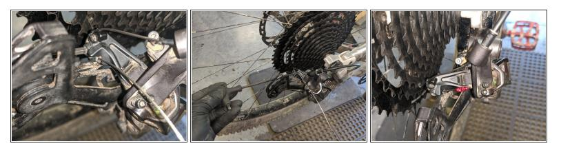
Before installing a new shift cable, inspect your shift housing closely. Dirty, abraded, worn, cracked, or otherwise-damaged housing should be replaced before proceeding.
