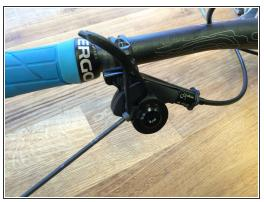
With the lever installed on the bike, adjust the paddle position to your preference and tighten the screw to 1N\*m
