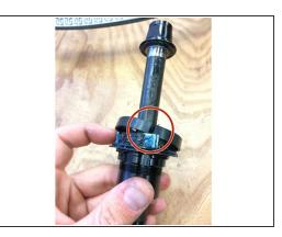
Pull the tab on the rubber ring, the ring will split at the slit and slide off the freehub body
