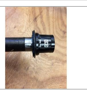
First, make sure the non-drive endcap seal is seated on the endcap as shown
