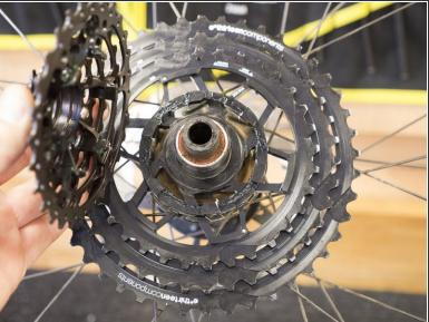
Once you have turned the cassette to the unlock position, remove the steel sprocket assembly from the hub.
