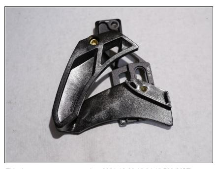
Start by loosening the upper slider bolt and opening the upper slider
