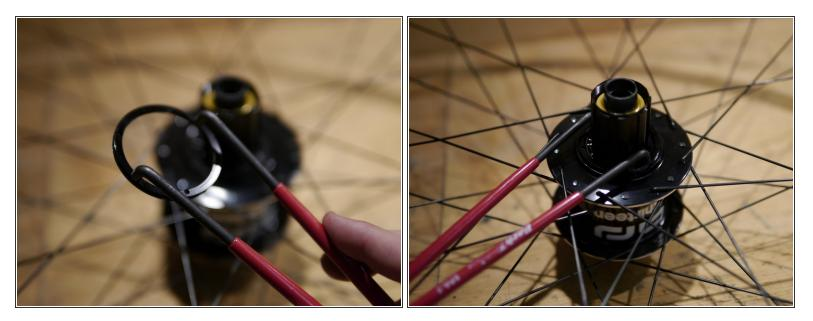
Put one drop of freehub oil on the rubber dust seal and install the freehub dust seal lockring
