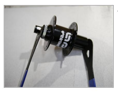
Loosen the non-driveside endcap by turning counter clockwise using cone wrenches
