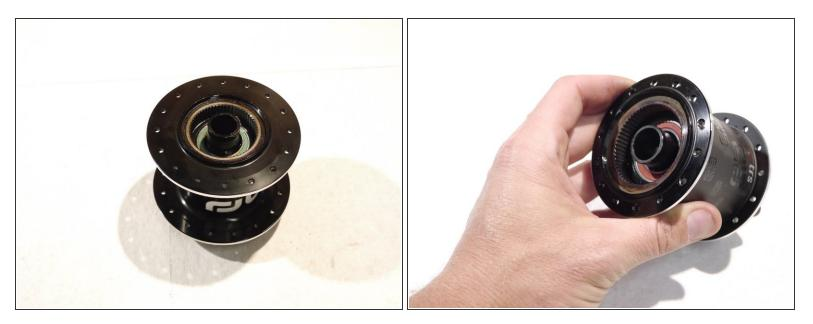
At this point the hub is most of the way apart, you can <u>service bearings</u>, replace worn parts or just <u>clean things up</u>
