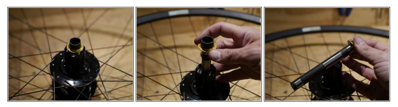
Slide the steel axle out of the drive side of the hub
