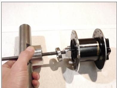
Remove the bearing from the hub shell
