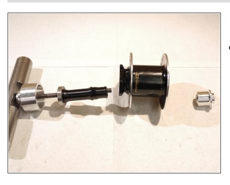
Remove the axle and bearing from the hub shell
