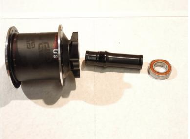
Remove the axle and bearing from the hub shell
