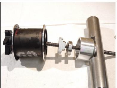
Remove the bearing from the hub shell
