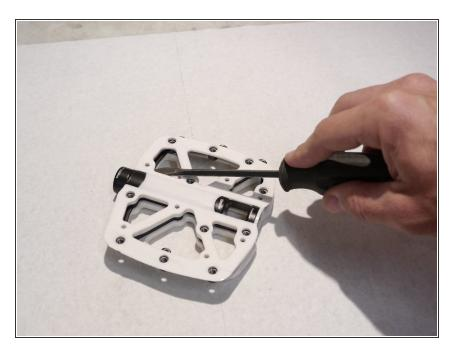
For older pedals it may be helpful to loosen the wearplate before removal by prying a corner up
