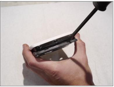
Newer pedal plastics include slots for a flat blade screw driver if you are having trouble prying the plates off
