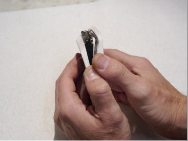
Once the pins are removed simply pry the wearplates off the pedal body
