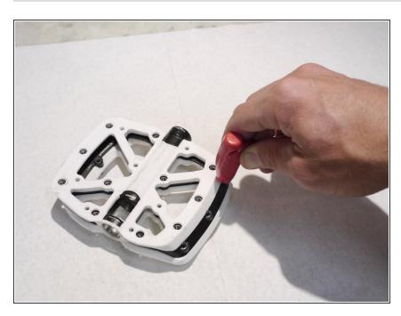
Start by removing all the pedal pins, these are accessed from the back of the pin
