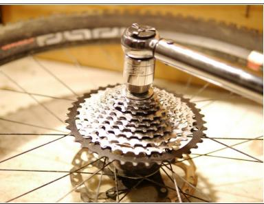
Lightly grease and install the cassette lockring and torque to spec.
