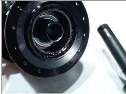
Slide axle and freehub assembly out of hub shell
