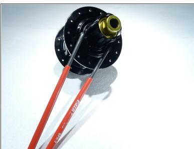
install the freehub seal lockring
