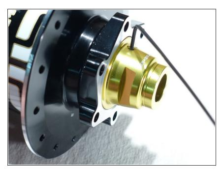
Loosen both 1.5mm grub screws on non-drive side endcap
