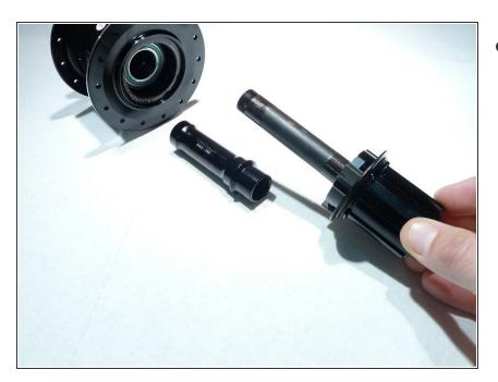
Remove the axle reducer
