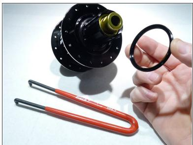
Remove freehub lockring by turning counter clockwise with pin spanner
