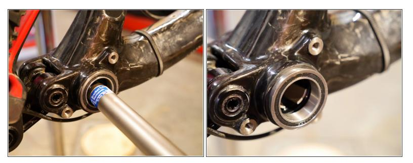
• To remove the BB cup, we recommend using a Park Tool headset cup removal tool
