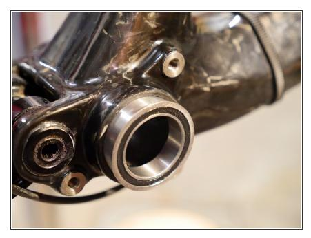
Slide the cup into the frame as far as it will go. It should just start to go into the frame.
