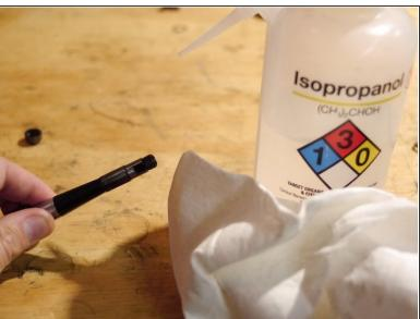
Clean the Igus bearings and bearing seats with denatured alcohol
