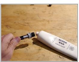
Install the seals on the Spin Control knob and axle and lightly grease using Rock and Roll Super Web Grease
