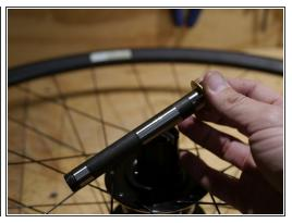
Slide the steel axle out of the drive side of the hub
