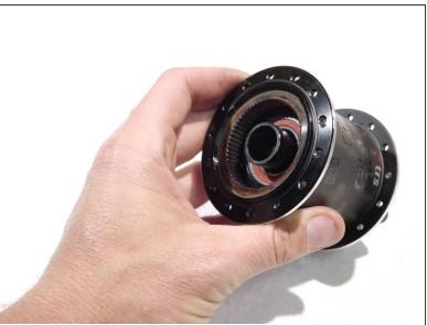
At this point the hub is most of the way apart, you can <u>service bearings</u>, replace worn parts or <u>just</u> <u>clean things up</u>
