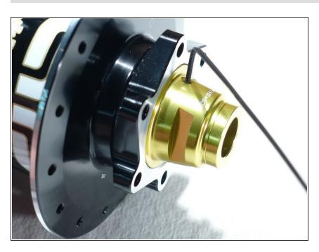
When you are happy with the adjustment, tighten the 1.5mm set screws to 1.5nm
