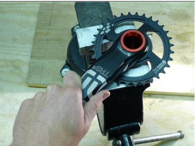
Press down on the driveside arm and spindle assembly to ensure that is does not slip in the tool
