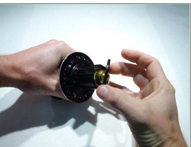
Remove freehub lockring by turning counter clockwise with pin spanner
