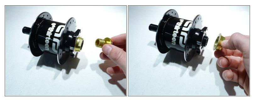
Loosen the preload ring by turning it clockwise
