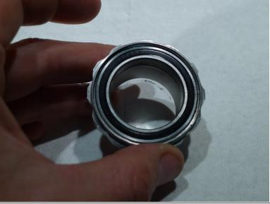
Replace the cartridge bearing seal by pressing it back into place by hand
