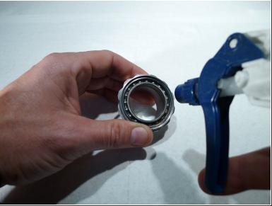
With the cartridge bearing seal removed, clean the bearing throughly
