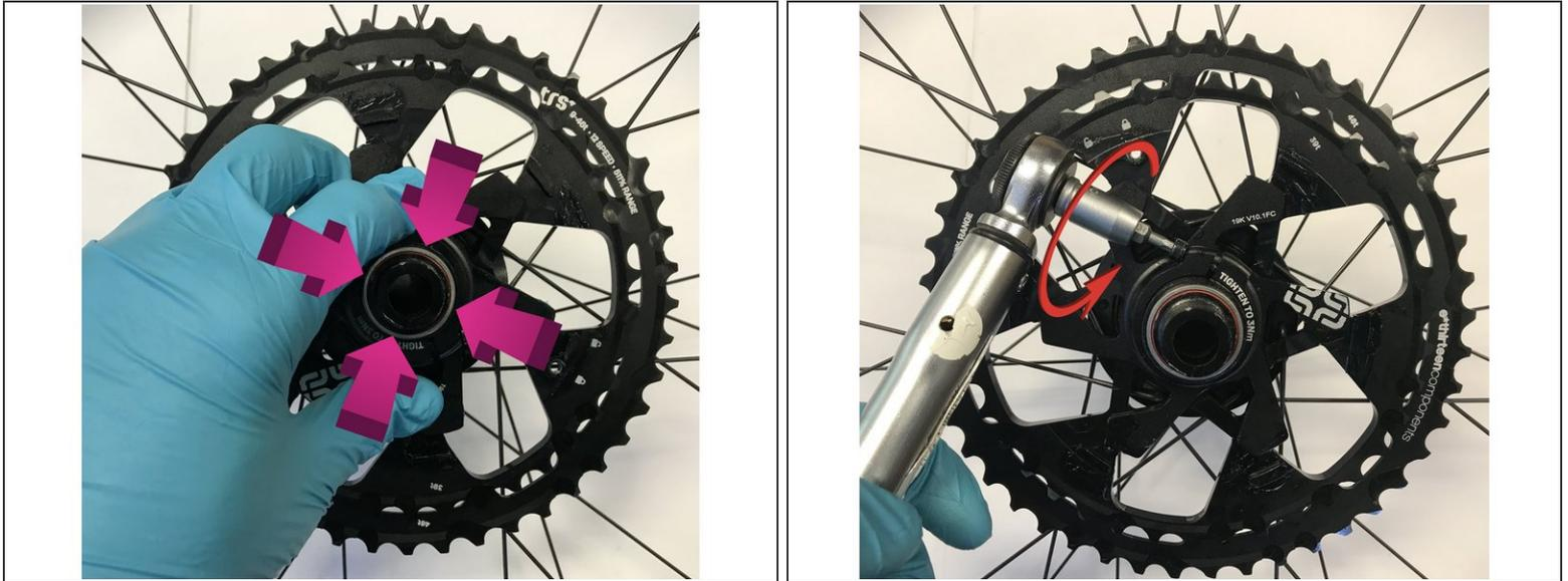
**⚠ NOTE: Special step for Hope hubs!! - If you are installing a pinch-bolt cassette on a Hope XD™ driver, you will need a special shim available free of charge from us. Please go to Step 3 BEFORE torquing the pinch bolt of the alloy section.**
