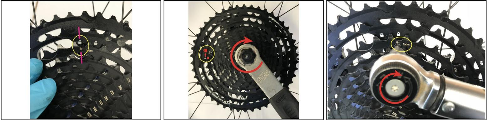
**⚠** Verify that the engineered plastic bushing is installed in the steel portion of the cassette. This piece is critical for the function of the cassette. The cassette will be damaged if it is not installed.
