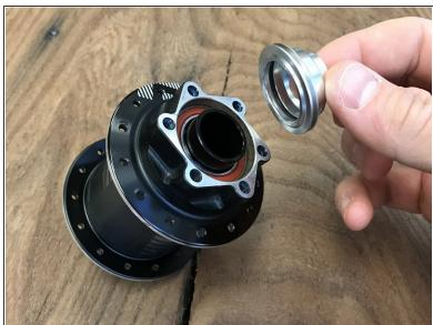
Any brand bearing press will work as long as the correct size bearing drifts are used. DO NOT HAMMER OUT BEARINGS - This can lead to a debonded hub shell.
