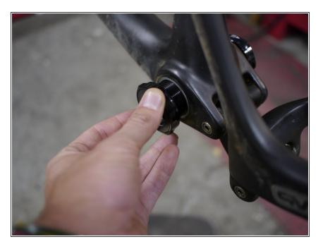
Install the non-drive side BB cup making sure the center tube is properly aligned
