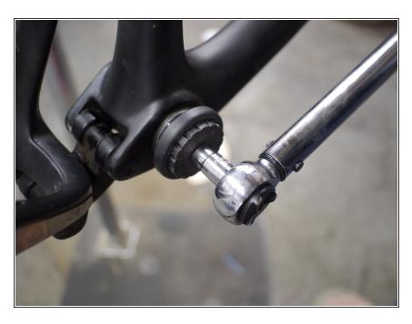
Using the e\*thirteen BB tool in conjunction with a 10mm hex bit and torque wrench, tighten the BB cup to 34-41nm
