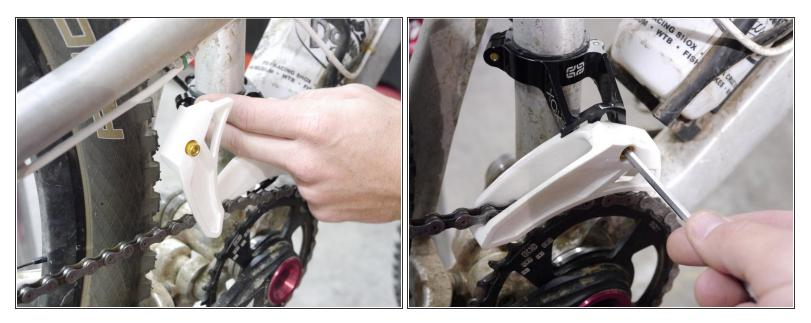
• Close the slider, lightly tighten the bolt
