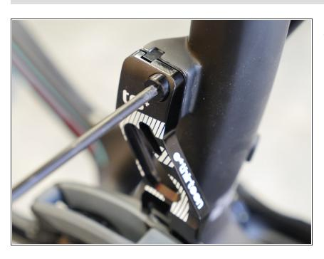
Tighten the fixing bolt to 6N\*m
