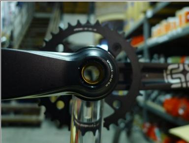
• Remove the crank fixing bolt with an 8mm hex wrench
