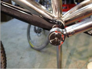
To remove cranks using a self extractor cap, simply turn the 8mm hex screw counter clockwise.
