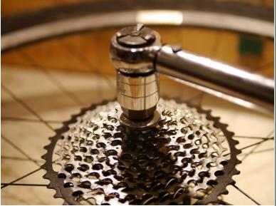
Lightly grease and install the cassette lockring and torque to spec.
