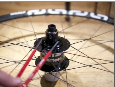
Install the freehub dust seal lockring (if used)
