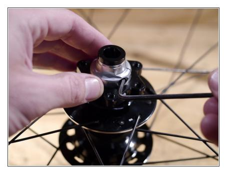
Loosen the 3mm hex endcap screw, by turning counterclockwise
