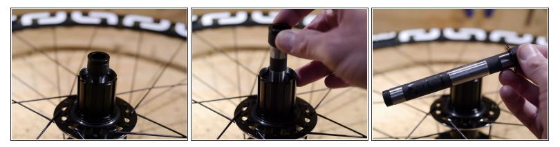
• Slide the steel axle out of the drive side of the hub
