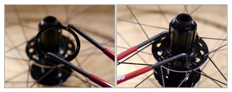
• Put one drop of freehub oil on the rubber dust seal and install the freehub dust seal lockring
