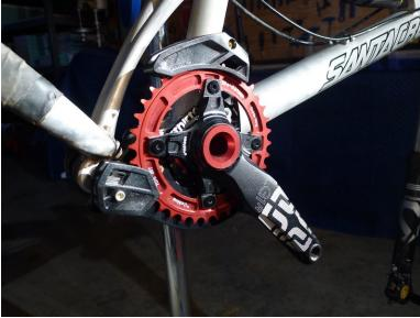
Reinstall the lower slider and adjust it into the proper chainring size position using the marks on the back of the bashguard, torque to 0.9nm
